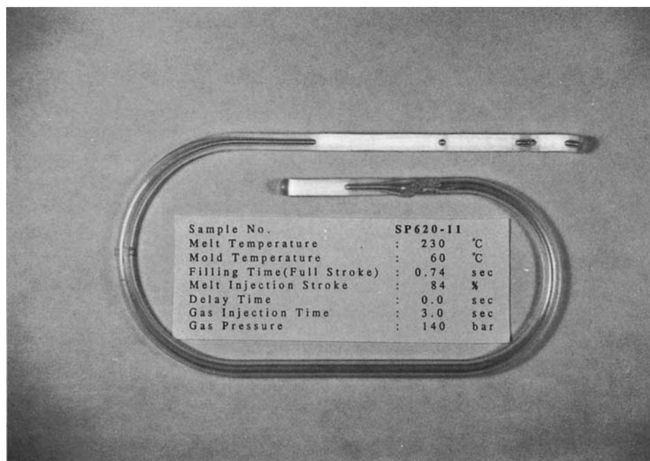
Figure 6 Gas-assisted injection-molded spiral tube.
